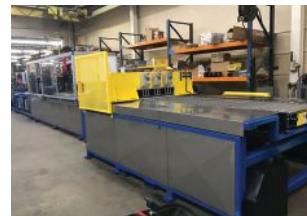
In line Cut-Off Saw Systems travels and cuts product at line speed
