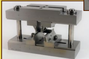
Three and Four Point Short Beam Flexure ASTM D 790, D 6272, D 7264, D 2344
